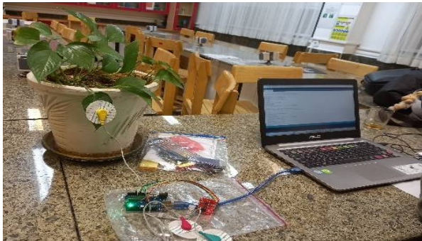
Figure 1: The experimental set up utilized for capturing plant electrophysiological signals
