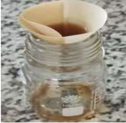
Figure 1: Removal of chlorophyll from the rosemary extract via activated charcoal treatment, demonstrating the visual color change from dark green to pale yellow/amber
