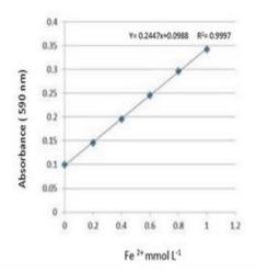
**Figure 1.** Linear equation resulting from different concentrations of the standard solution
