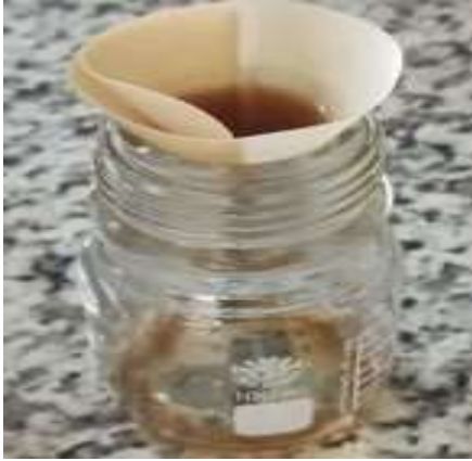
Figure 1: Removal of chlorophyll from the rosemary extract via activated charcoal treatment, demonstrating the visual color change from dark green to pale yellow/amber
