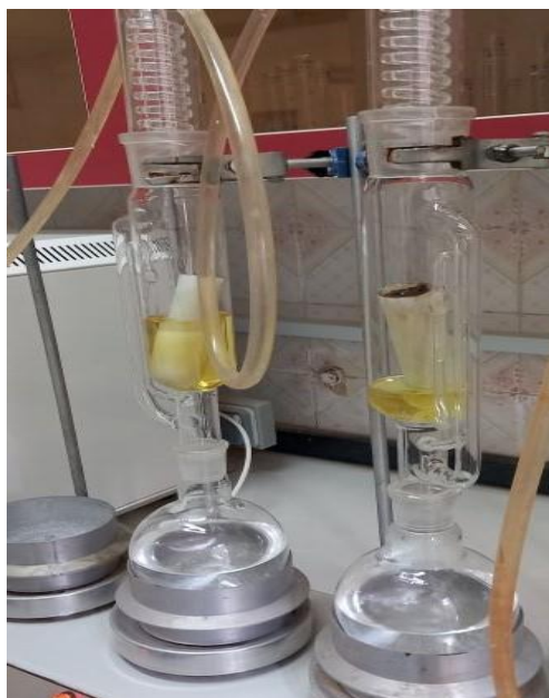
Figure 3-3: Extraction of wild pistachio fruit using a Soxhlet apparatus.
