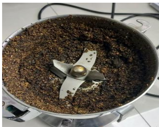
Figure 3-2: Wild pistachio fruit ground using a laboratory mill.
